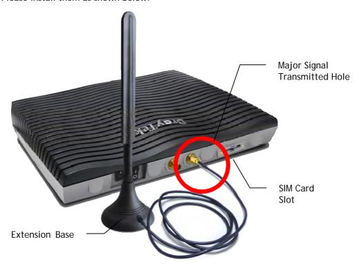
Note, if only one antenna shall be installed, please use the mounting hole (major signal transmitted hole) near to the SIM card slot.
