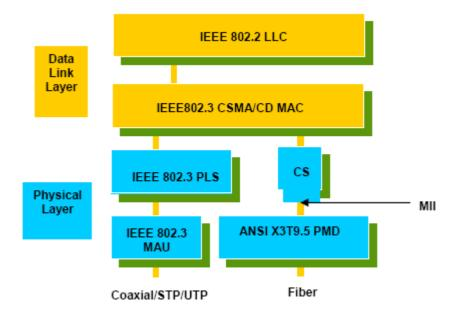
This above diagram shows the Ethernet architecture, LLC sub-layer and MAC sub-layer, which are responded to the Data Link layer, and transceivers, which are responded to the Physical layer in OSI model. In this section, we are mainly describing the MAC sub-layer.
