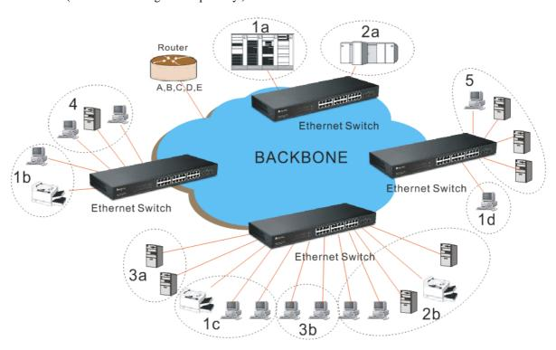
Now we apply VLAN technology to configure the system shown as the figure above. We can partition the users into the different logical networks which have their own broadcast domain. The traffic will not disturb among these logical networks. The users 1x (x denotes  $a \sim d$ ) are members of VLAN 1. Any traffic within VLAN 1 does not flow to VLAN 2 and
