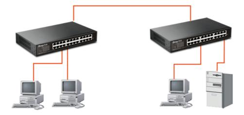
If VLAN is enabled and configured, each node in the network that can communicate each other directly is bounded in the same VLAN area.
