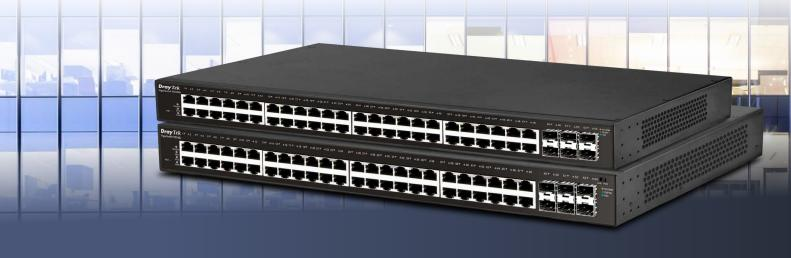
DrayTek VigorSwitch 2540x series is a Layer 2+ Managed 10 Gbps switch with 48 Gigabit Ethernet ports and 6 x SFP+ 10Gbps Fiber links. Supporting advanced Layer 3 features, DHCP Server and VLAN Routing. Moreover, it supports VLAN routing to route the inter-VLAN traffic directly, shares loads of the router, and improve overall network performance.
