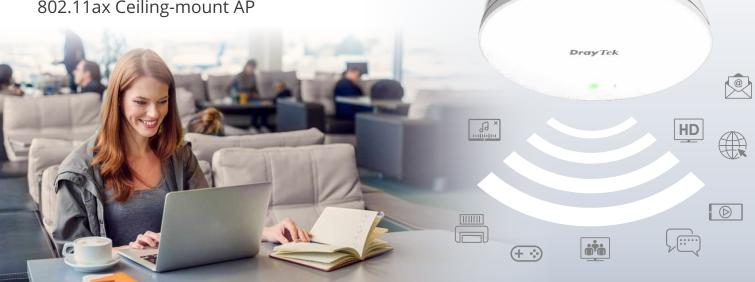
VigorAP 960C is an 11ax ceiling-mount wireless access point. With wire-liked speed up to 1.2 Gbps in 5GHz band and 600Mbps in 2.4GHz, it's suitable for high density environments. It can be cloud-managed by VigorACS, and also act as the mesh Root AP to manage up to 7 mesh node APs in LAN.
