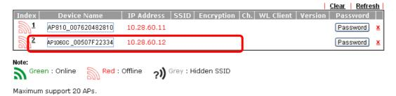
When AP Devices connect via another intermediate router or switch, please check/unblock the following ports UDP:67,68,4944 and TCP:80 of the router/switch, thus AP status can be retrieved.
