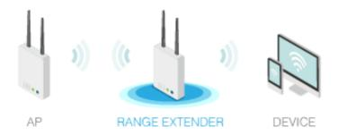
The access point can act as a wireless repeater; it can be Station and AP at the same time. It can use Station function to connect to a root AP and use AP function to serve all wireless stations within its coverage.
