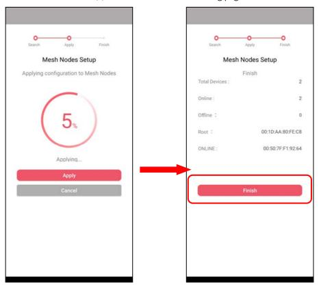
7. A network with mesh root and mesh node has been set up successfully.
